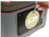
Mount camera to mounting plate. Rotate 4. camera until text on back is parallel to top of IsoPlane.
